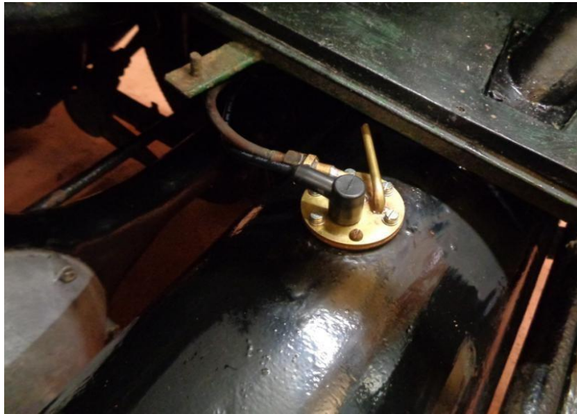
Re-installed tank with new sender unit fitted
