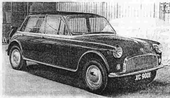
Alvis shape echoes SII Oxford (top rt); XC9001 (left) drew on suspension of Alvis and engine was half its V8
