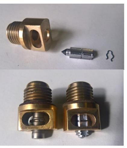
Altering a jet by drilling or reaming will change the flow characteristics and may cause a jet to have a very unpredictable flow curve relative to intake air speed.
