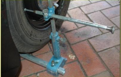
As can be seen in the above photos the centre line of the wheel is the starting point for the measurement. I repeated the process this time without rotating the wheels in order to see if the rims were true and they were. Assuming that all adjustments have been done correctly and everything else is in proper order the steering wheel spokes should be symmetrical in the straight ahead position.
